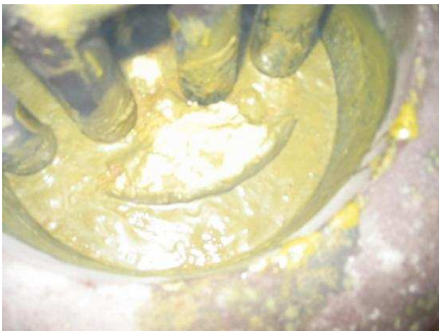
Sulphur Melted using Thermic Fluid (No Steam)
